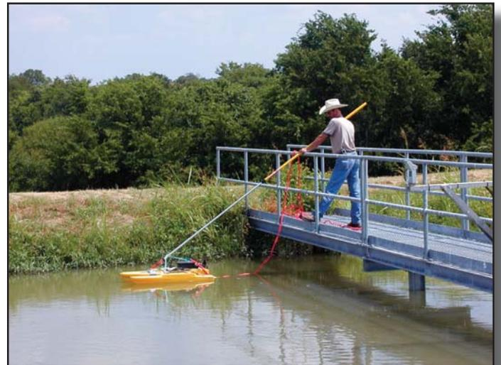
*David Murdoch of the Lower Colorado River Authority deploys a trimaran-mounted RiverSurveyor to measure flow throughout the vertical water column. In obstructed reaches, the instrument's stationary software delivers excellent data to a simple, intuitive interface, says Murdoch's colleague, Keith Ging.*
