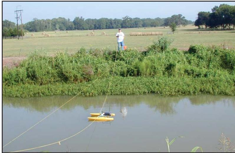
*A Lower Colorado River Authority hydrologist remotely directs a catamaran mounted RiverSurveyor along a transect across a canal. Along a transect or using stationary software, the RiverSurveyor uses Doppler sonar to quickly, accurately measure flow in the vertical water column.*
