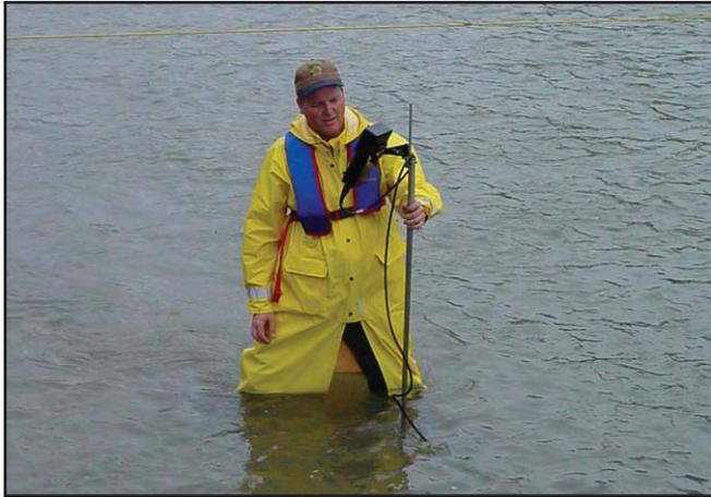
*John Roberts of the Lower Colorado River Authority's Hydromet Operations Group used FlowTracker acoustic Doppler velocimeters to conduct a study of water discharged from one of its dams, checking hydroturbine ratings. The group also used the FlowTrackers to study fresh water inflows from groundwater – vital information for exploring a proposed interbasin water sharing plan, and for managing the LCRA's extensive system.*
